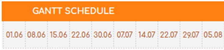
That means the entire duration of the project is divided into 40 equal time intervals and the start date of each period is showed in the header of the chart columns. In the example on the screenshot, one division equals a week.
